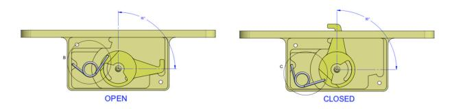
The huge advantage of using a torsion spring is that its influence is always 'live' - that is, initially it exerts a force against the turning of the key - gradually increasing until it reaches the half way 'tipping' point when it takes over and snaps the locking arm to the opposite state. Once experienced, nothing else will do ...
