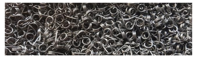
The twin coil torsion springs produced specially for the *smart*Lock to my design are precision made and shot-peened - a process used to strengthen and extend the life of high end components used in formula 1 and other high stress environments.
